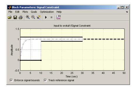
Before running the optimization, change the function tolerance to 0.01 within the Options dialog box. This ensures that the new objective function meets the imposed tolerances. To do this, open the Options dialog box by selecting **Optimization > Optimization Options** from the menu in the Signal Constraint window and then change the **Function tolerance** value to 0.01 within the **Optimization Options** pane of the Options dialog box, as shown in the following figure.
