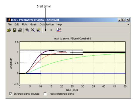
The blue line shows the initial response and the black line shows the current, or final, response. As you can see, the final response signal lies within the constraint bounds.
